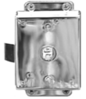
Latch #21.709-25; 25 mm backset brass chrome plated 7 x 7 mm spindle
