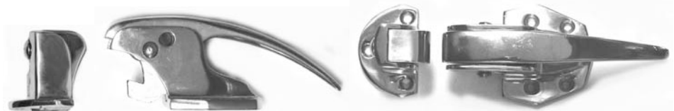
#88.066 Latch for up lay doors with 1/2 inch offset; stainless steel , with padlock provision Base 2 5/16 inch x 2 3/16 inch" Strike sold separate #88.067 Strike for offset adjustable 5/8 x 1 1/4 inch
